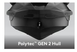
Specifically designed to meet the needs of recreational riders, the Polytec GEN 2 material is highly robust and scratch-resistant, and reduces overall vehicle weight to improve efficiency.
