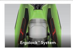
A narrow seat profile with deep knee pockets lets riders sit naturally and use the leg muscles to hold onto the machine for more control.
